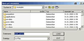
Select a path and a file and click on the **LOAD** button to load the file to the *Thales* software. Click on the **Display Diagram** icon on the POL main page to display the data in a graphical form.
