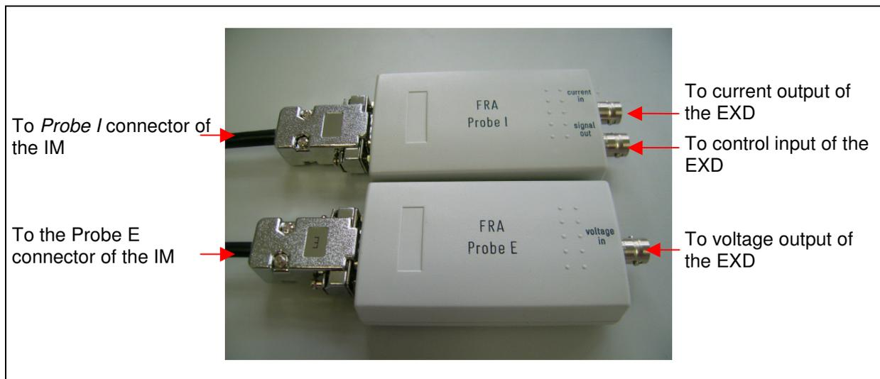
The FRA module interfaces third-party potentiostats and electronic loads to the IM6/Zennium system. The EXD must provide an analogue control input and analogue signal outputs for the measured current and voltage. FRA is fully supported by the Thales software. Only the gain factors have to be set for each EXD individually.
