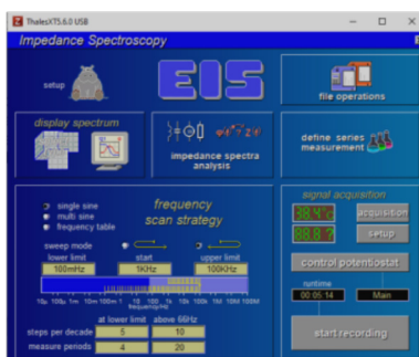
2. Input desired EIS parameters & click on “control potentiostat”
